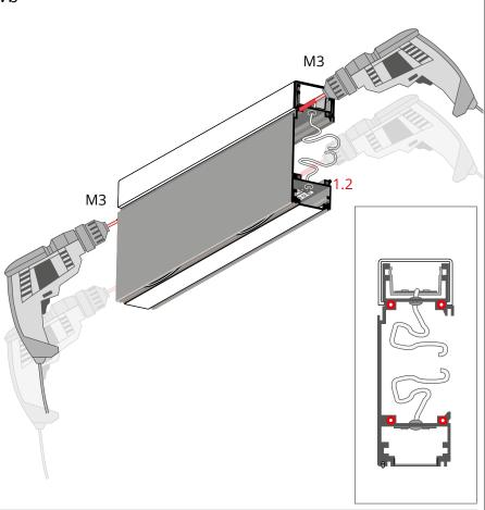
Thread the marked channels of the item (1.2) from both sides with the M3 screw
