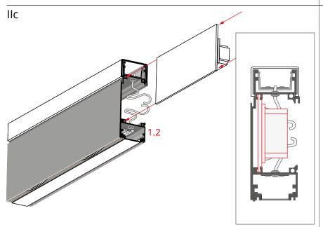
Put the mounting pad with the power supply in the channels in item (1.2) and slide the whole assembly into the profile.
