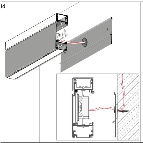
Connect the 230 V / 120 V cable to the power supply.
