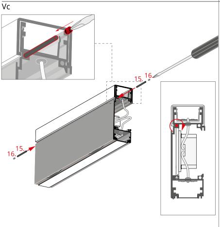
Put the previously-cut rods (15) into the channels from both sides of the profile and tighten them all the way with pressure screws (16).
