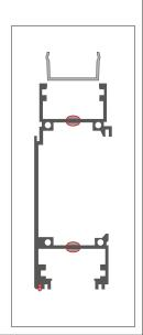
Mount the glands (7) in the holes. Place the springs (8) in the grooves in the lower section of the profile.
