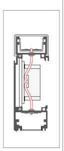
Connect the cables from LED strips to the power supply.
