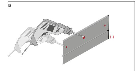
Drill the holes in the item (1.1) of the KIDES-DUO profile. Note the diameters of the side holes may need to be adjusted to accommodate the screws and middle hole may need to be adjusted to accommodate the 230 V / 120 V cable.
