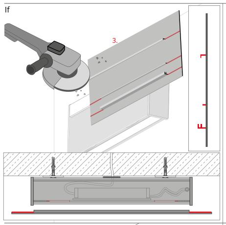
Grind the hooks off the ATRA profile (3) to the length that will allow to mount it on the KIDES-DUO profile with the previously mounted end caps.
