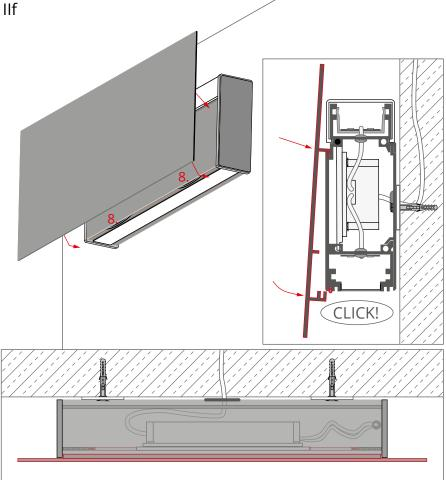
Put the ATRA profile on the KIDES-DUO profile as shown in the drawing. Springs (8) will secure the ATRA profile against falling off.
