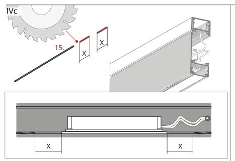
Measure the distance from the mounting insert to the end of the threads in the channels. Cut the two sections from the plastic rod (15), matching the measured length.
