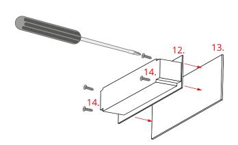
Mount the power supply 12 V / 24 V (12) to the mounting pad (13) with screws (14).
