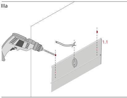
Drill screw holes in the wall on both sides of the 230 V / 120 V cable. Their position should reflect the holes in the item (1.1).
