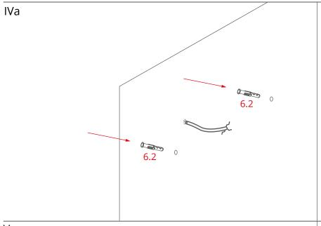
Put the wall anchors (6.2) into the pre-drilled holes.
