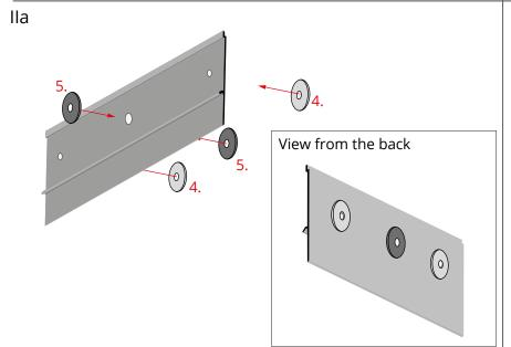
Adhere the gaskets (5) to both sides of the middle hole. Adhere the washers (4) to the back side of the profile on the screw holes.
