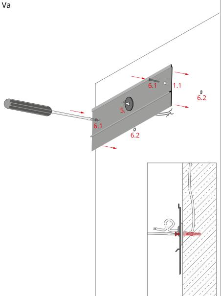
Lead the (230 V / 120 V) cable through the gasket. Then screw the item (1.1) to the wall with the use of screws (6.1), using the holes drilled on the sides and the wall anchors (6.2).
