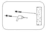
1. Drill holes into the mounting surface and insert expansion screws
