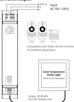
40W Color Temperature Panel Light Driver Model No.: PL2 40W RGB+CCT Panel Light Driver Model No.: PL5
